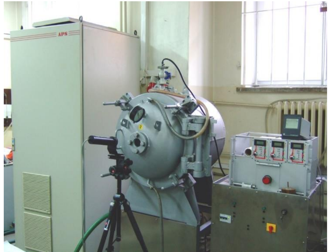
TECHNOLOGICAL STAND FOR GLOW DISCHARGE SURFACE LAYER PRODUCTION DEVELOPED BY MATERIAL ENGINEERING DEPARTMENT OF WARSAW TECHNOLOGICAL UNIVERSITY
