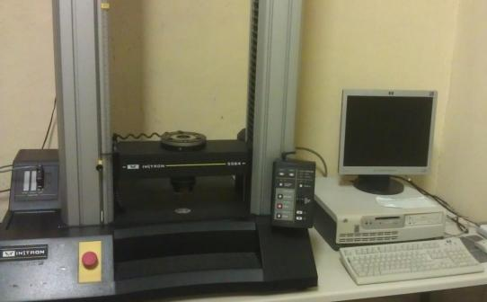
The native chordae has been isolated from the fresh specimen excluding any portion of leaflets and papillary muscle in order to avoid any influence of these remnent on mechanics of native chordae. For the same reason we used an highly efficient and selective pneumatic branching device to eliminate any influence of point of connection between native or synthetic chordae to the Instron.
